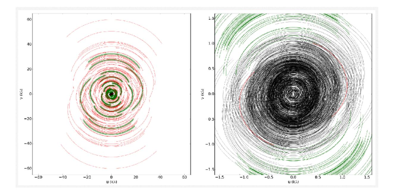
The uv-coverage of the LOFAR core + remote stations gives high angular resolution (6" at 140 MHz or 15" at 50 MHz) combined with excellent surface brightness sensitivity for recovering very extended emission.
