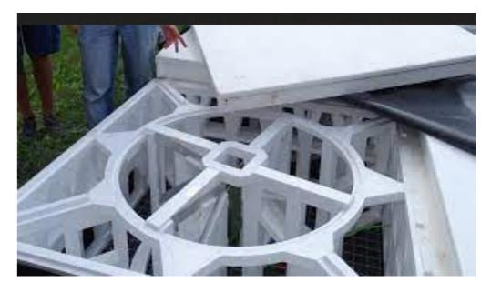
LOFAR **High** (110-250 MHz) **band antenna.** Core ones are 24 antenna arranged with 30.8m diameter, remote ones are 48 antenna with 41m diameter, international ones are 96 antenna with 56m diameter.
