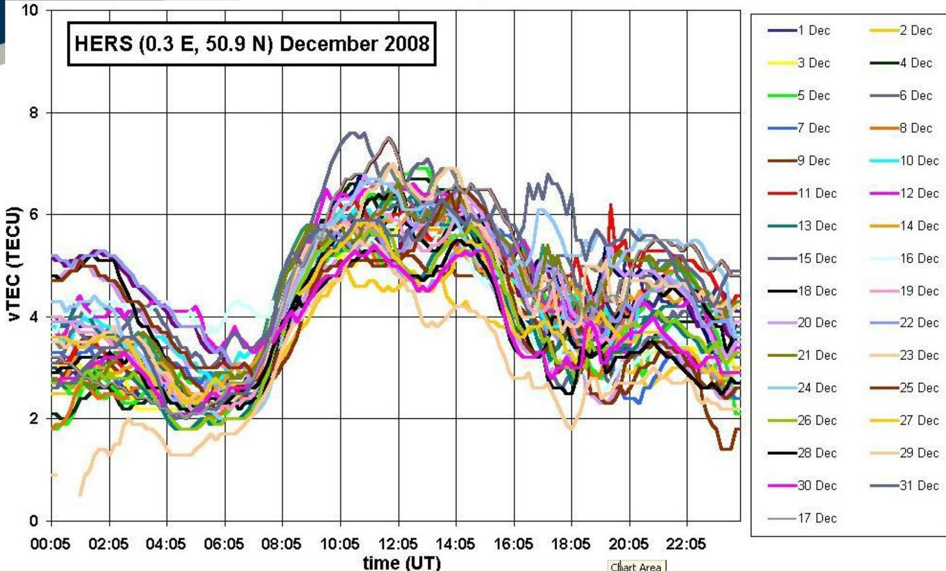
Plot of the **vTEC** diurnal variations over a mid-latitude ground-based GPS receiver at **HERS, UK** during **absolute solar minimum** in December 2008 when **Ri=0.8**.
