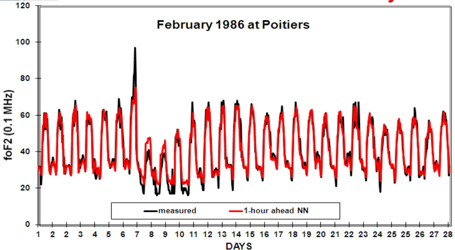
Measured and 1-hour ahead forecast *foF2* values at *Poitiers* ( $46.6^\circ$  N,  $0.3^\circ$  E) ionosonde station in *February 1986*.
