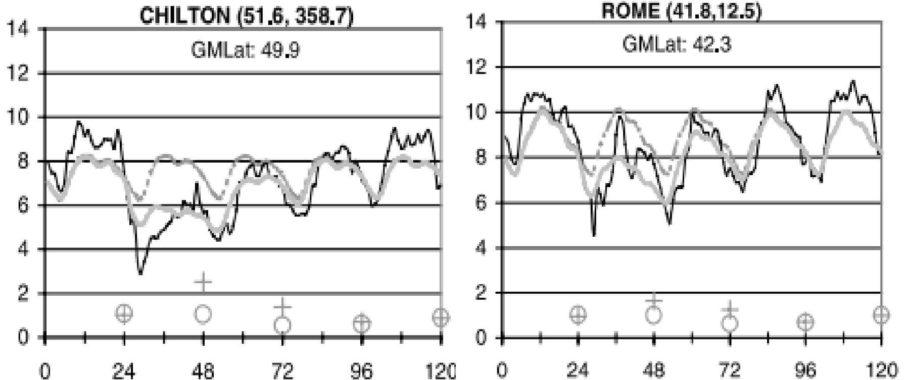
Data and output of the *IRI95* and *IRI2000* models at two different locations for the 23 - 27 May 2000 storm. The dashed shaded line shows *IRI95*, the solid line is the observation, and the solid shaded line shows *IRI2000*.
