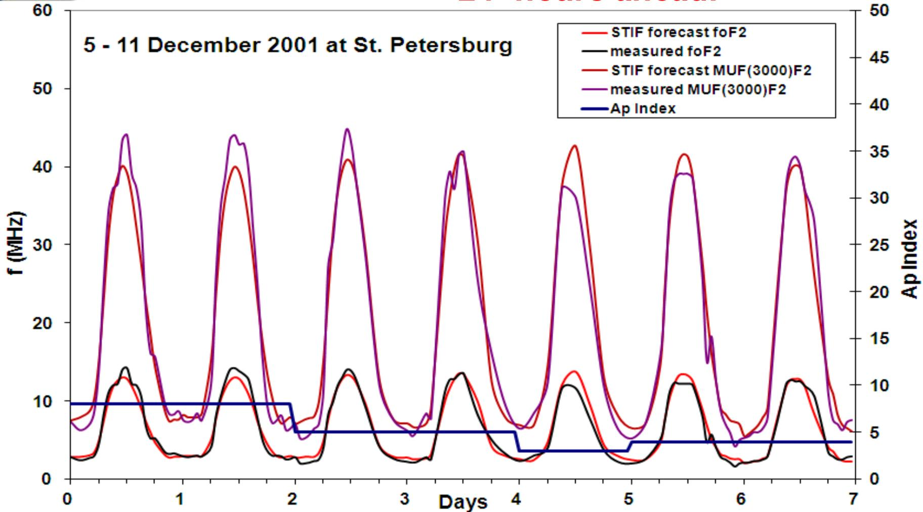
Typical STIF foF2 and MUF(3000)F2 results and measurements at the St Petersburg (59.9° N, 30.7° E) ionosonde station during quiet geomagnetic conditions.
