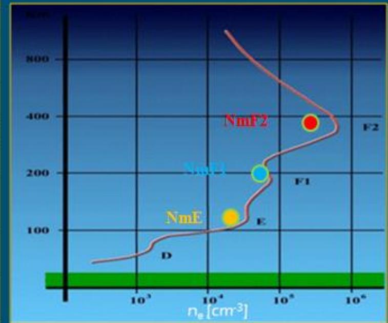
The maximum electron density  $N_M$  corresponds to the maximum reflected incidence frequency called the critical frequency  $f_o$
