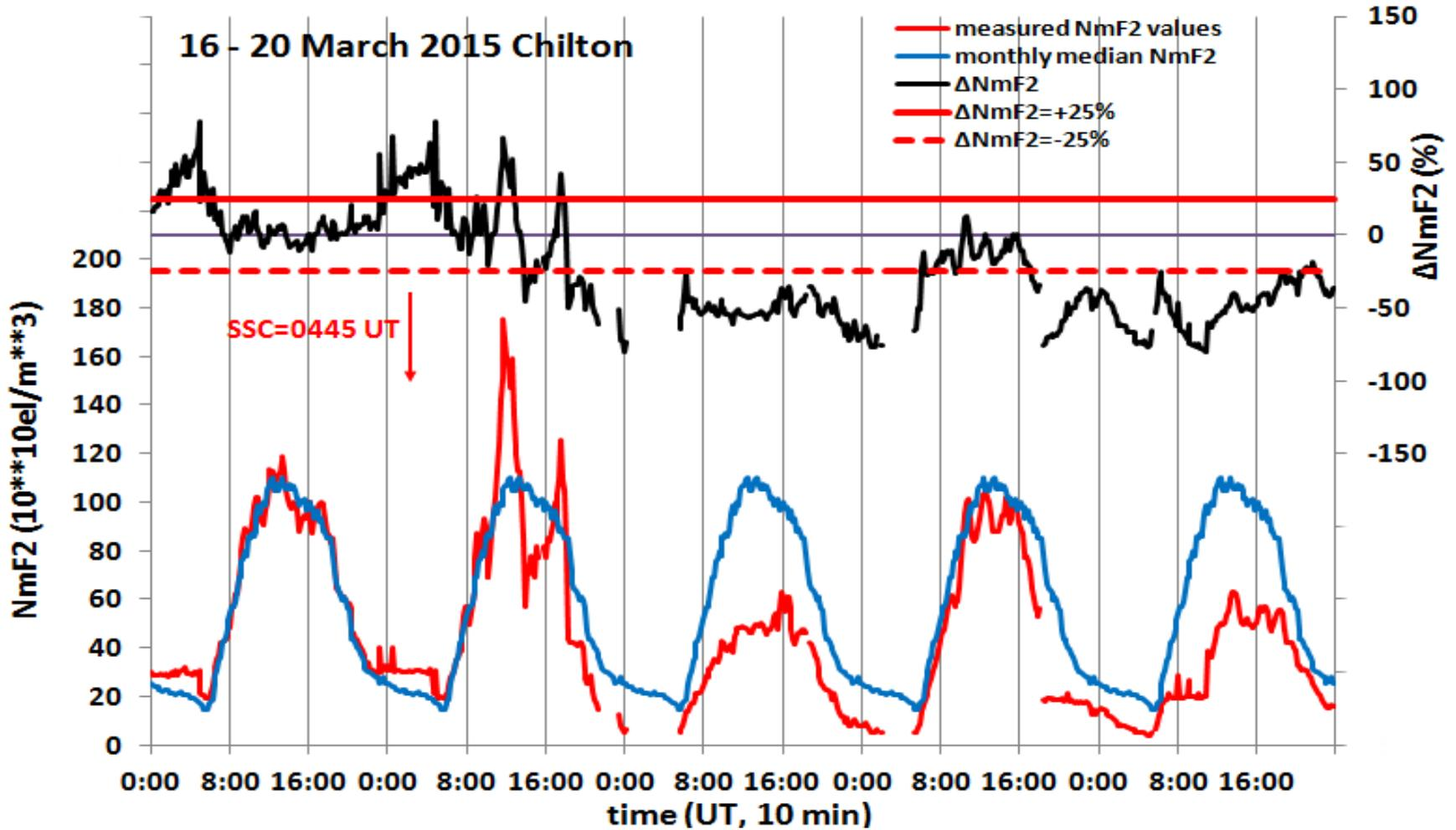
***NmF2 values and their percentage changes from the monthly median  $\Delta NmF2$  for Chilton ( $358.67^\circ \text{ E}$ ,  $51.70^\circ \text{ N}$ ) ionosonde station.***
