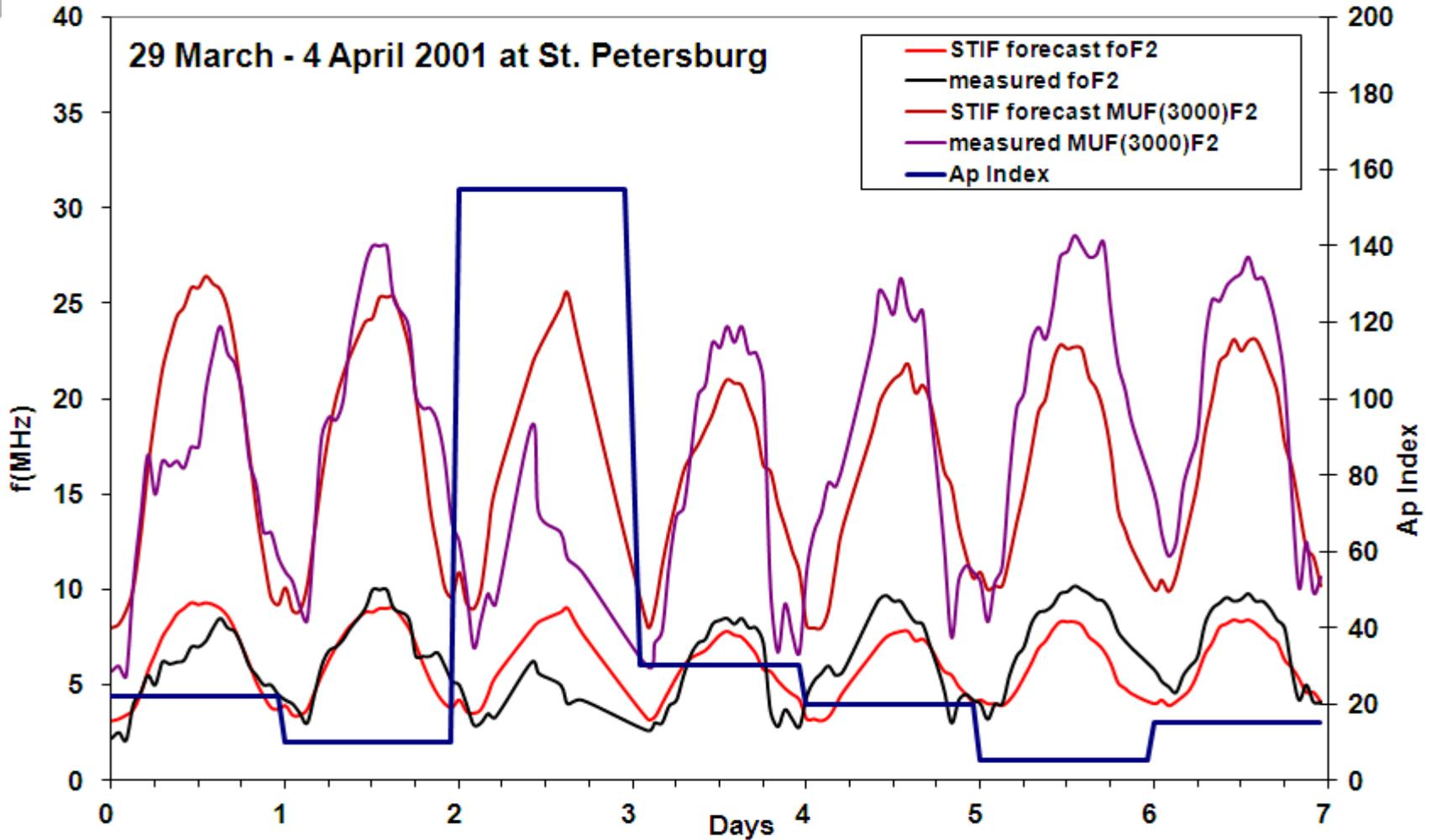
Typical STIF  $foF2$  and  $MUF(3000)F2$  results and measurements at the St Petersburg ( $59.9^\circ$  N,  $30.7^\circ$  E) ionosonde station during disturbed geomagnetic conditions.
