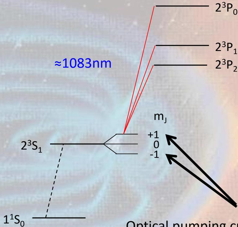
Optical pumping creates an imbalance in these two metastable energy levels, which depends on the field direction
