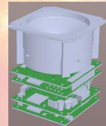
Measures spectral and angular distributions of ~3–70 keV/q ST ions at ~60 s resolution.
