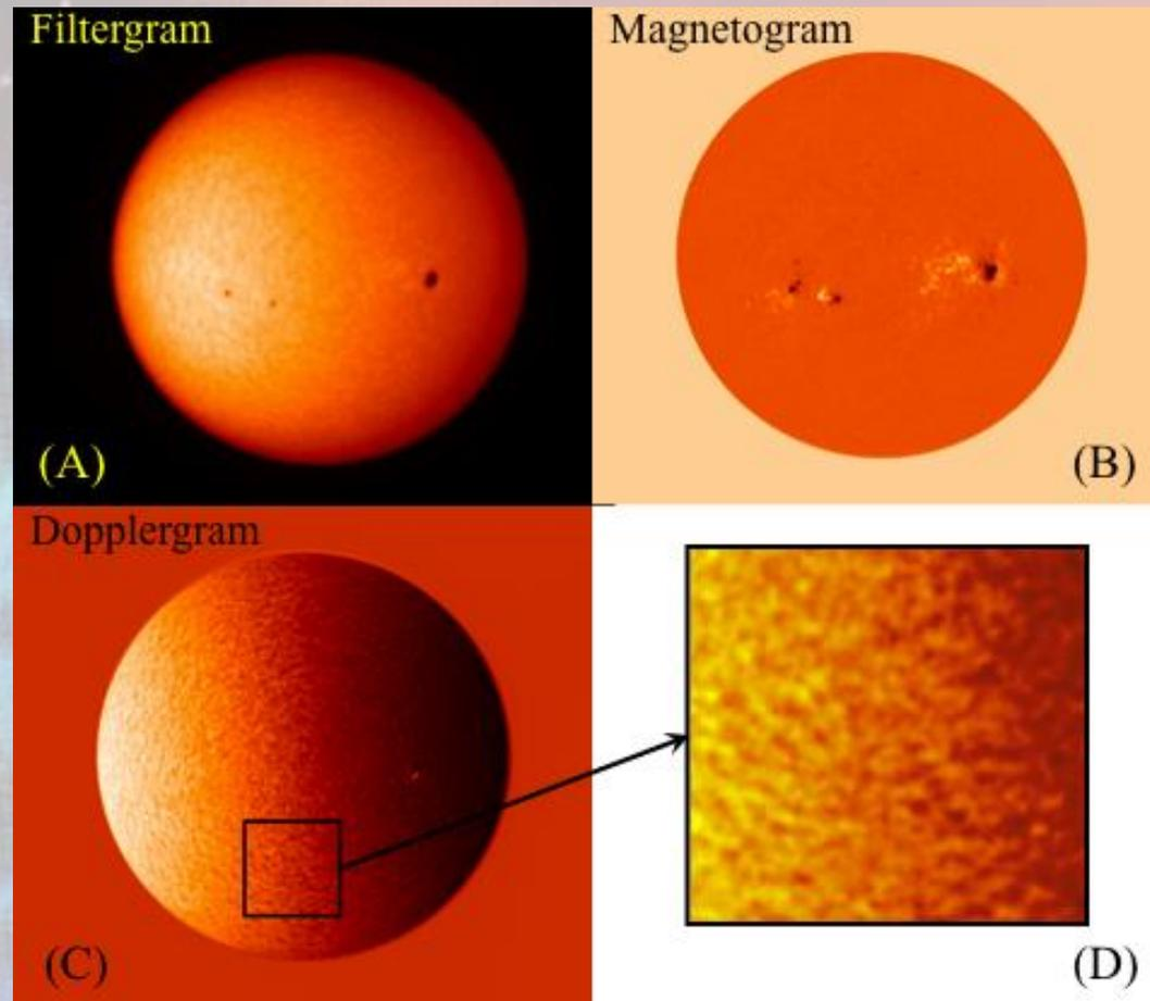
Panel A) shows an image of the sun, through a single MOF passband, B) shows an image of the net circular polarization, ie a magnetogram, C) shows a normalized difference image between the two passbands, which is proportional to Doppler shift - a Dopplergram.
