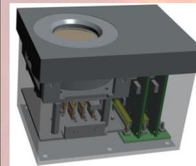
Measures ~100 keV–3 MeV electrons, ~2–40 MeV/n protons and He, and ~5–150 MeV/n C-Fe at 60 s resolution
