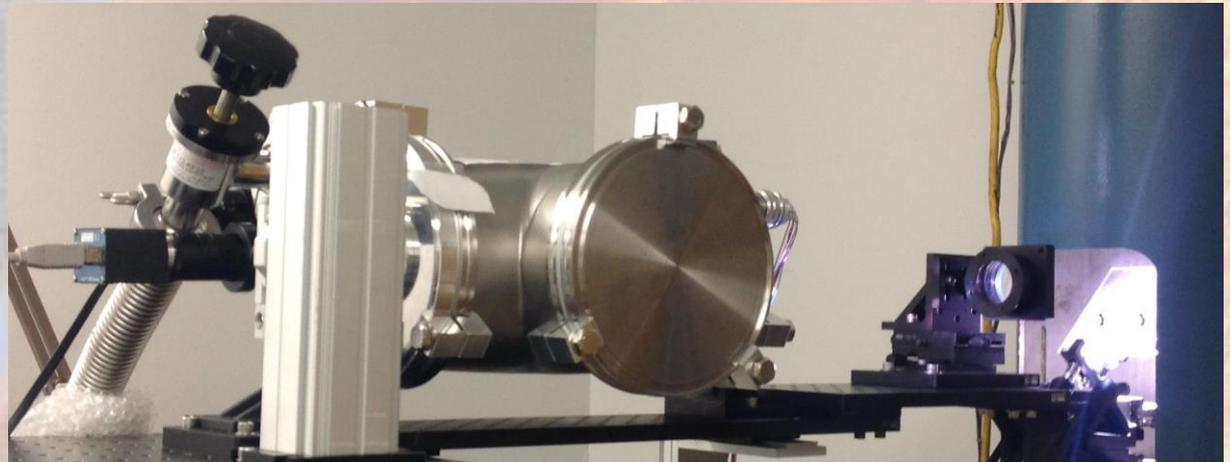
Used for verifying thermal models and power consumption in vacuum, testing performance. Limited vibration testing already completed
