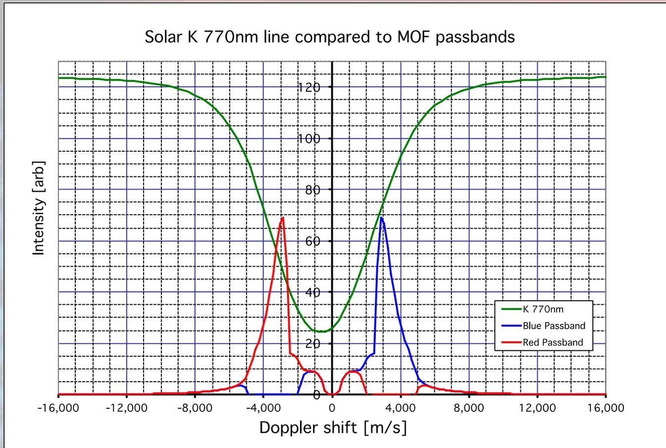
Red and blue Doppler Imager pass-bands, compared to the K 770 nm solar absorption line. Intensity ratios are proportional to Doppler shift, circular polarization is proportional to the line-of-sight magnetic field
