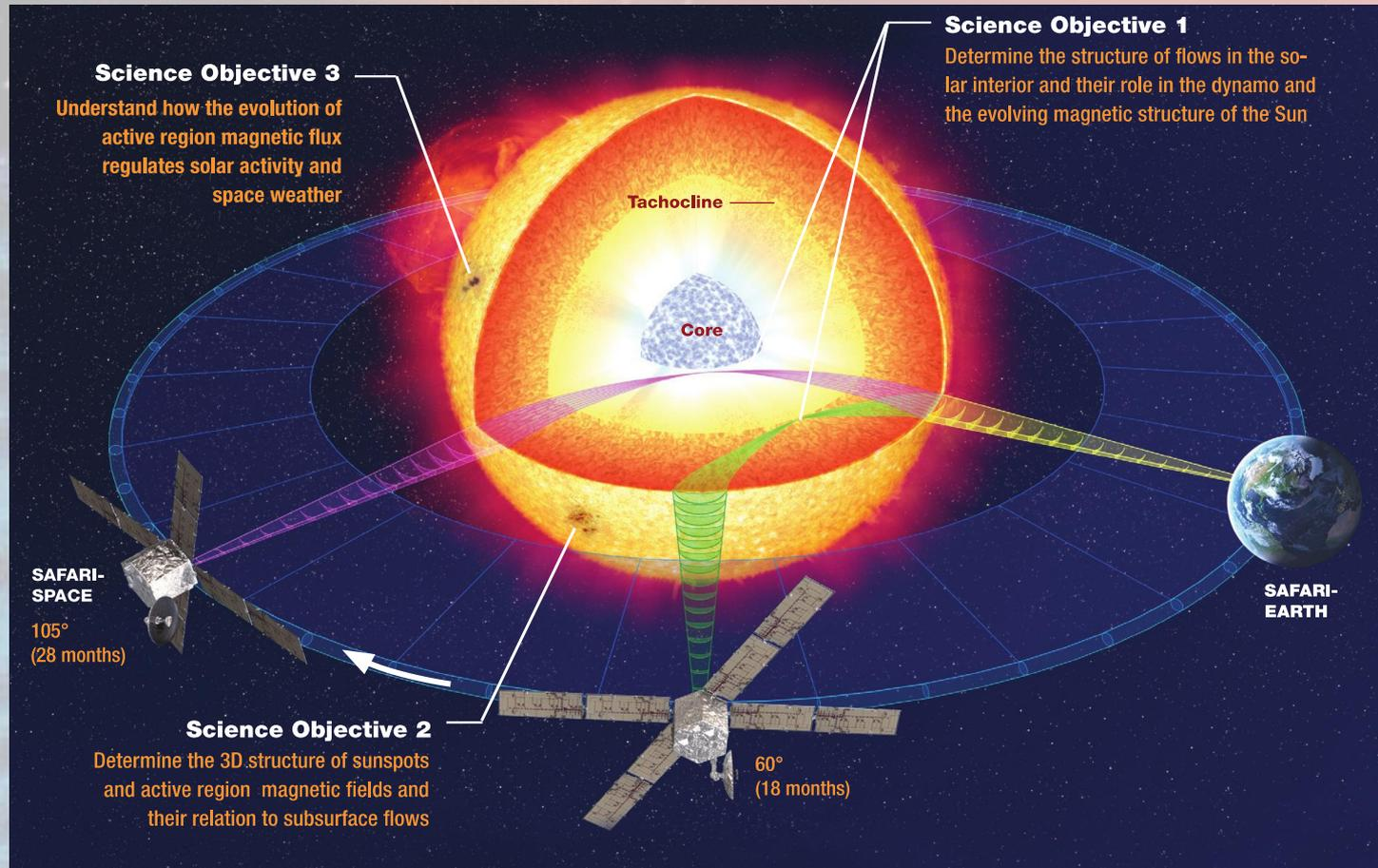
An overview of SAFARI – by making helioseismic and magnetic measurements from two vantage points – one on the earth, we can probe the deep interior of the sun, measure transverse flows in the photosphere, and make stereoscopic magnetic field measurements
