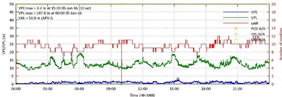
**SDV - Performance Analysis Diagrams : Vertical Stanford Diagram**
