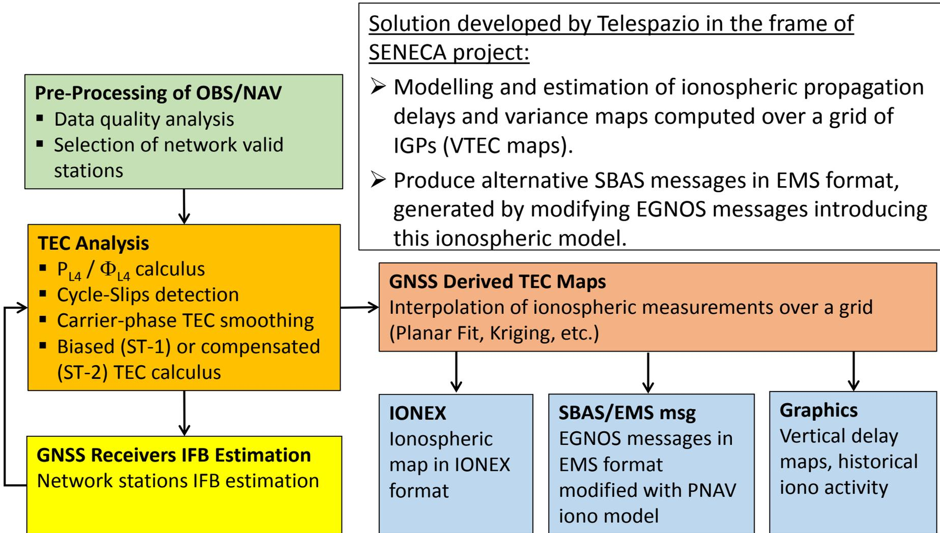
Solution developed by Telespazio in the frame of SENECA project:
