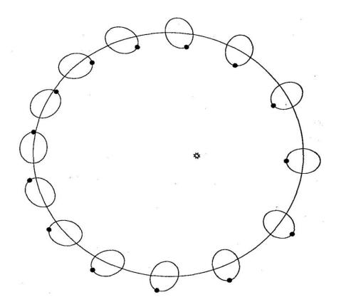
Mercury is now in a 3:2 spin-orbit resonance with orbital eccentricity of ~0.2.
