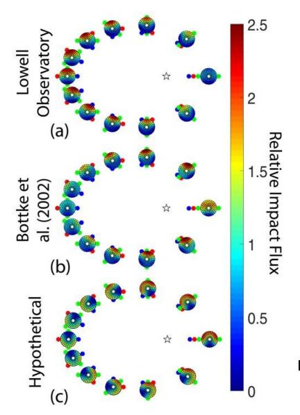
The impact dynamics on Mercury for substantial eccentricity (*e*=0.4 for left figures).
