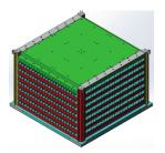
The BGOcal (60  $cm \times 60cm \times 35 cm$ ) is composed of 14 layers (7 for the *x*-coord., 7 for the *y*-coord.), and it is ~ 32  $X_0$  deep. This depth ensures that almost 100% of the energy of  $e^{\pm}$  and  $\gamma$  is deposited in the calorimeter (~ 40% for hadr.). Each crystal is read out by 2 PMTs, mounted on both of its ends. In order to cover a large dynamic range (2 × 10<sup>6</sup>), the signals are collected from 3 different dynodes
