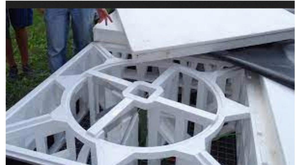
LOFAR **High** (110-250 MHz) **band antenna**. Core ones are 24 antenna arranged with 30.8m diameter, remote ones are 48 antenna with 41m diameter, international ones are 96 antenna with 56m diameter.
